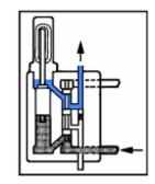
4. Maintained lower supply line pressure forces the main piston to the uppermost limit of its travel, delivering the full measured charge to the bearing. Beyond this point, maintaining lower supply line pressure will have no effect.
