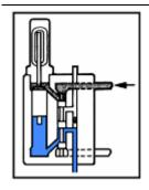
Pressurisation of the upper supply line forces the inlet piston down, thereby un-covering both diagonal passages. Lubricant passes through the upper diagonal passage into the main chamber and acts on the top of the main piston, causing it to move.
