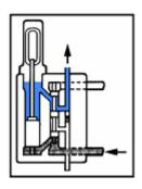
Pressure is switched to the lower supply line (on a signal from the flow directing valve) which forces the inlet piston up, thereby uncovering both diagonal passages. Lubricant passes through the lower diagonal into the main chamber and acts on the bottom of the main piston, causing it to move upward.
