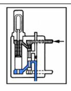
Maintained upper supply line pressure forces the main piston to the lowest limit of its travel, delivering the full measured charge to the bearing. Beyond this point, maintaining upper supply line pressure will have no effect.
