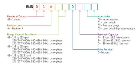
The BM-B Lubricator features a smart part number ordering system, where you can tailor the pump to meet your needs. First, choose the number of outlets, revision level, flange mounted gear motor, drive position, reservoir capacity and accessories you need. Then, put the numbers into the corresponding squares in the easy-to-use grid. You now have the customized part number.
